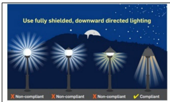
Figure 2. Light Fixture Standards.
